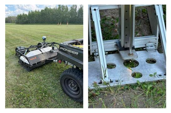
A Mala Mira HDR Multi-Chanel Ground Penetrating Radar machine being towed across search area (left), and an S4 Subterra Gray Soil Spectroscopy machine (right) during a ground search in 2024 (Office of the Independent Special Interlocutor).
