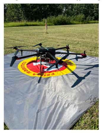
A FEMIA Robotics D20 Drone with Riegl Lidar Sensor VUX-120 during a site search in 2024 (Office of the Independent Special Interlocutor).
